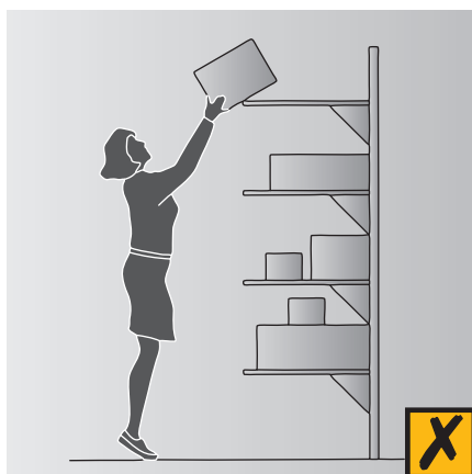
Figure 4.17 Shelving too high and deep
