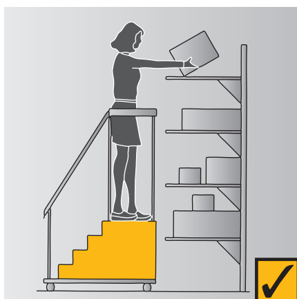
Figure 4.18 Controlling risk of storage at height
