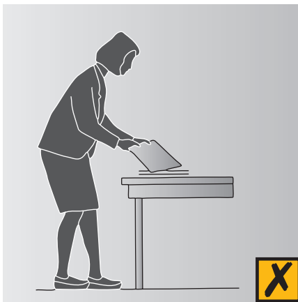
Figure 4.8 Incorrect standing-height bench
